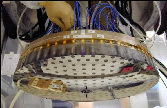
The MMT adaptive secondary built by the U. Arizona and Arcetri : 336 voice coils equipped at the back
