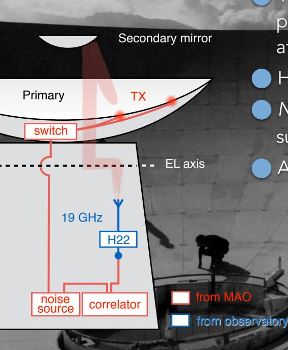
Top-level science requirement: High-accuracy phase measurement with  $\sigma(\theta) = 1 \text{ deg r.m.s.}$ at 20 GHz, corresponding to 40 µm r.m.s. H22 receiver *N*-element ( $N \ge 5$ ) 20 GHz transmitters on the surface of the 45 m primary Accelerometers
